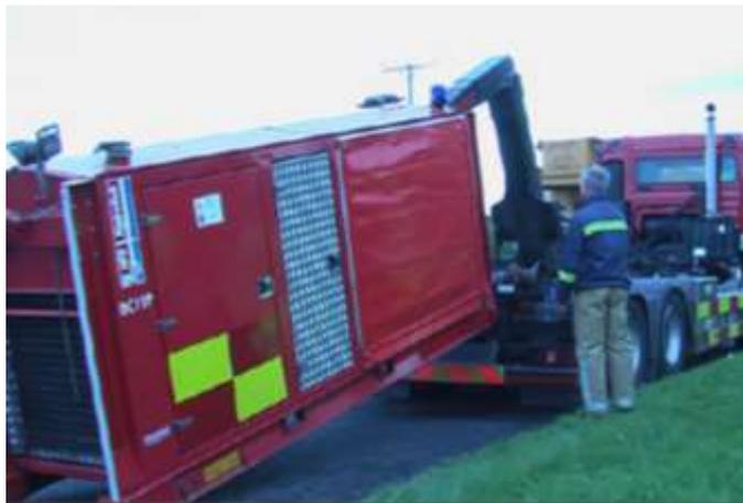
An example of an High Volume Pump for open water supply being used for firefighting operations.
